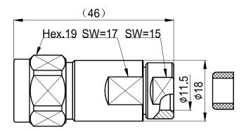
N Straight Male Connector for 3/8" Super Flexible RF Cable
