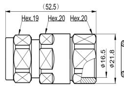
N Straight male Connector for 1/2" Flexible RF Cable
