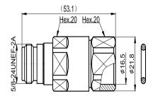
N Straight female Connector for 1/2" Flexible RF
